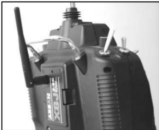
Mount removable antenna and screw it into the connector at the back of ASSAN's X8 2.4GHz RF Module. Finger tight only.
