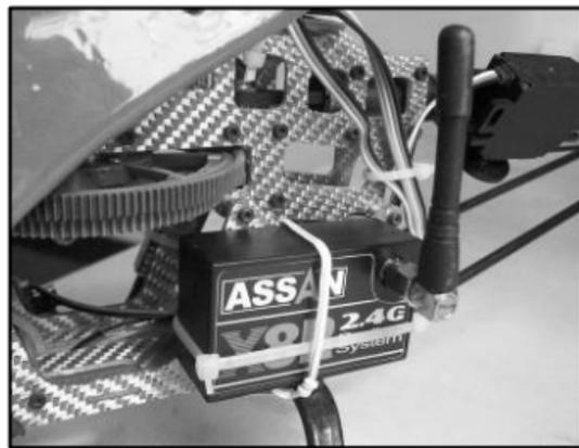
Screw out the red plastic cap on the antenna base in counterclockwise direction. Screw the 2.4GHz antenna pin into receiver base in clockwise direction. Finger tight only to avoid damage to the threads. The connector of antenna is universal one. The antenna should point outwards during use.
