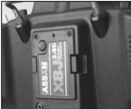
Take 2.4GHz RF model out of the package (X8F/X8J). Do not install the antenna first. Be careful not to damage the exposing part of screwing threads on antenna base.
