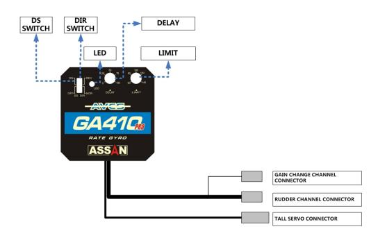
1. DS SWITCH: The ON position is for high speed signal Digital servo only
