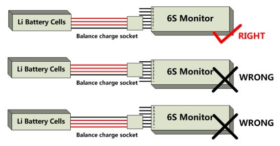
• **Display:** When connecting to the balance charging socket of the lithium battery pack, the voltage monitor will start measurement and display right away. It will display the voltage of the whole pack as well as each of the cells in a recurring manner. The display of "Axx.xx" implies that the total voltage is xx.xxV, while the display of "1c x.xx" or "2c x.xx" implies that the voltage of a cell is x.xxV.
